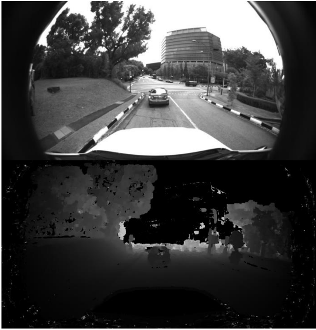
Figure 3. Original image (top) next to depth map (bottom). Depth values are invalid beyond a certain range, most noticeably for the building and road in the background of this image.
