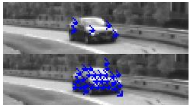
Figure 2. Feature points from algorithm (top) and manually added (bottom). Many feature points are required, even spread across the object, for accurate shape estimation.
